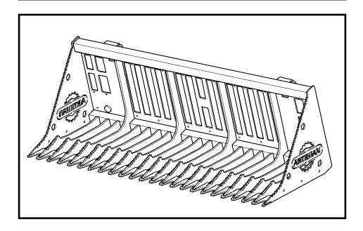
The Artillian Rock Bucket is designed to allow a compact tractor to lift, transport, or remove rocks from 2 inches or larger and sift out sand, dirt or other smaller debris.
