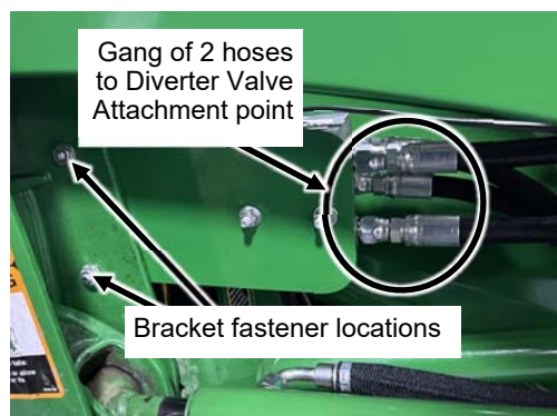
Fig. 2.a (Attach First Gang of Hoses to Valve)
