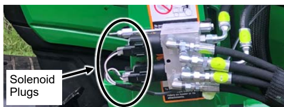
Fig. 4 (Attach Wire Harness Plugs to Solenoids)
