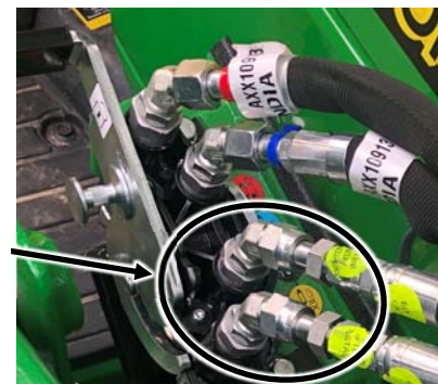
Fig. 3 (Disconnect Dump/Curl Hoses from Single Point Hydraulic Connector)
