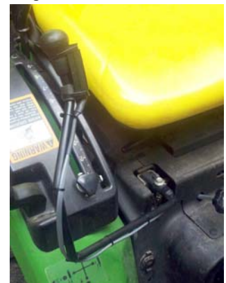
Diverter Valve Switch Install (Actual Loader Joystick May Vary from Image)
