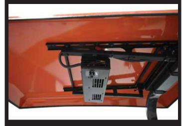
Fan is adjustable up to 45° in relation to the canopy. Overhead console gives easy access to blower speed controls and adjustable air vents.
