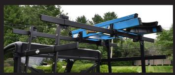
The tool "racks" mount to the vehicle bed using metal brackets embedded within the frame, with two Bars on each side of the bed and additional storage structure over the bed.
