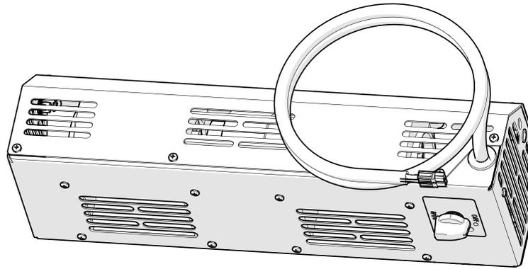
**NOTE:** The fan may be attached to the canopy frame while it is still on the tractor, however it may be easier to unlatch the canopy from the tractor to install the fan.
