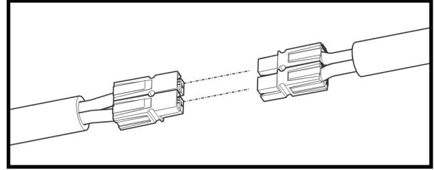
Fig. 4 (Connect Power Harness to Fan)
