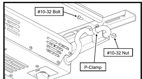
Fig. 3 (Attach Fan wire to Canopy frame)
