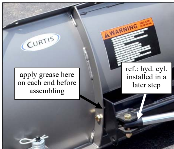
Fig. 1.1—Trip Frame to Moldboard
