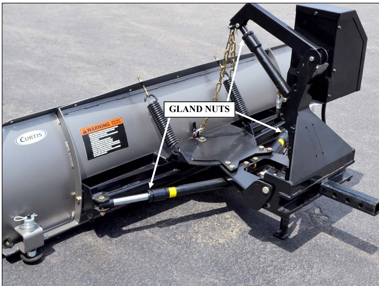
Fig. 11.3 repairing a Hydraulic Cylinder leak
