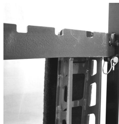
6. Latch Safety Wires on Pins (both ends)
