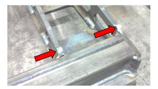
As a bare steel weldment, these frames ship with an anti-corrosive surface treatment. This coating does not affect weldability and can be wiped, washed or brushed away when ready for finishing.
