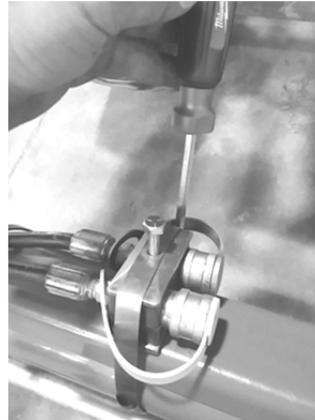
Dismantle the entire Single Port Manifold but **keep all parts**. Everything will be reused except for the manifold body components (shown below).
