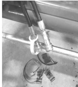
Set the Splitter Manifold on the loader torsion tube and screw the band clamp together loosely. Position the left end of the manifold approximately where the existing hoses end.
