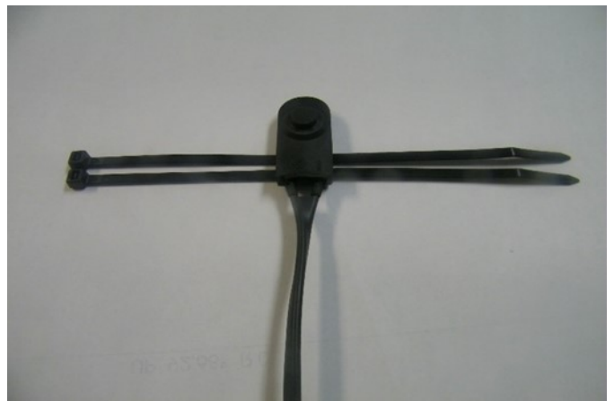
Rubber switch w/o a plastic housing
