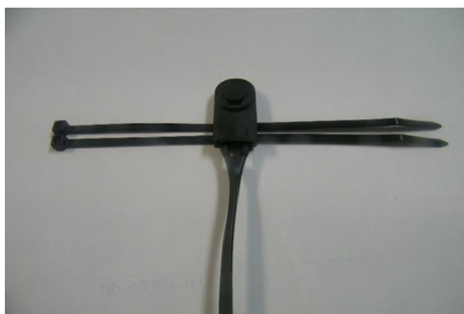
Rubber switch w/o a plastic housing
