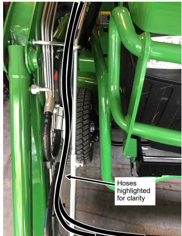
Fig. 3 (Route Gang of 4 Hoses up Loader)
