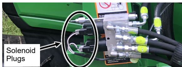
Fig. 5 (Attach Wire Harness Plugs to Solenoids)
