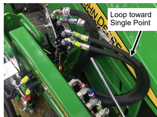
Fig. 3 (Loop Gang of 2 Hoses toward Single Point)
