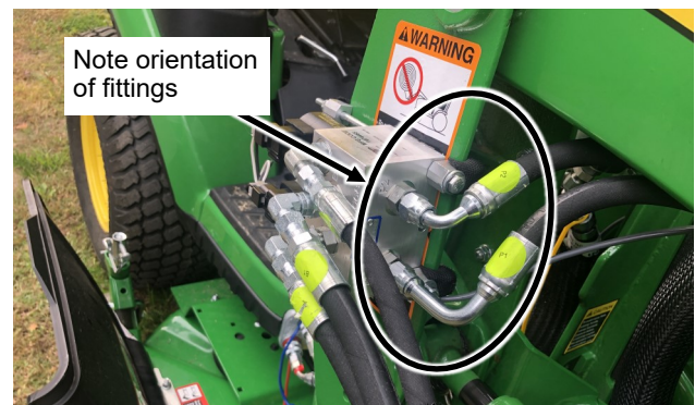
Fig. 2 (Attach Gang of 2 Hoses to Valve)
