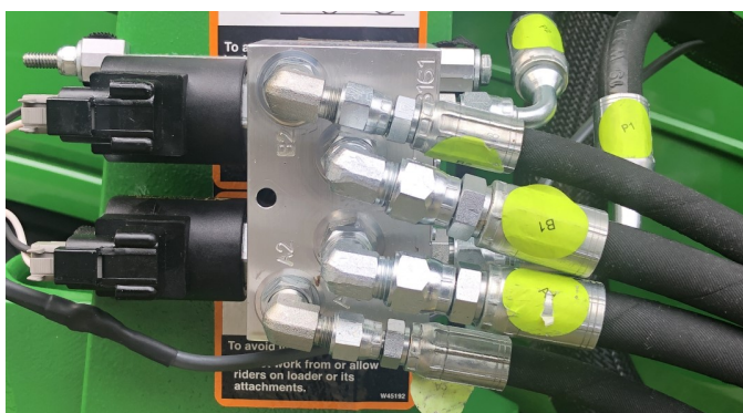
Fig. 7 (Connect Hoses to Diverter Valve)
